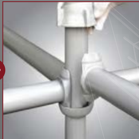
2. Lower the upper cup down the standard and rotate.
